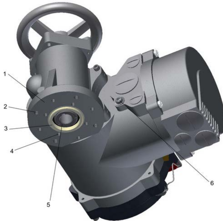
Figure 21: 1... mounting flange, 2... bore pattern G0/F10, 3... centring ring, 4... bore pattern F07, 5... shaft connection, 6... ground connection
